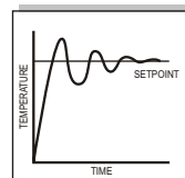
Figure 4 : Proportional and Integral Control Characteristic
