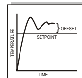
Figure 3 : Proportional Control Characteristic
